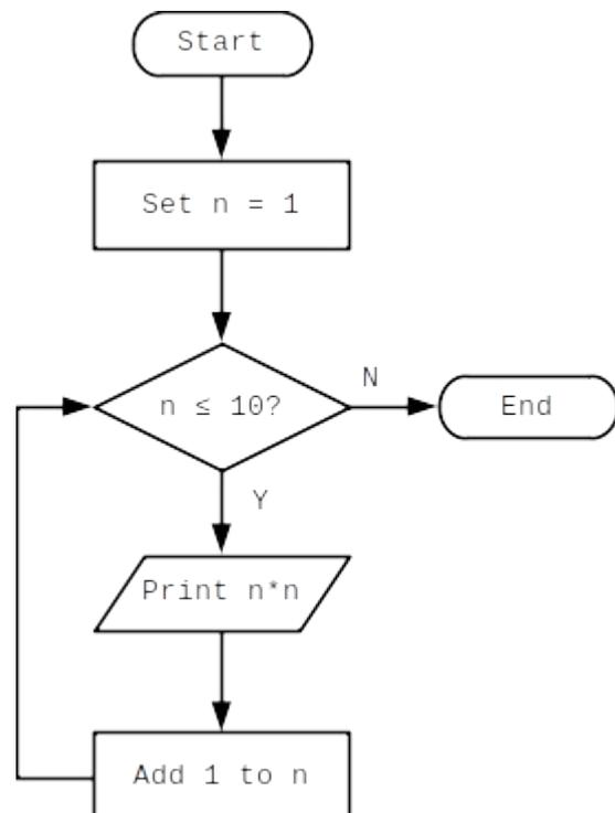
There is exactly one START and one END in this flowchart. The two PROCESSES are setting a counter and incrementing the value of the counter by one. A DECISION occurs when comparing the value of the counter to 10. If the value is less than or equal to ten, then the algorithm OUTPUTs the square and increments the counter. If not, then the algorithm ENDS.
