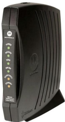
A cable modem
