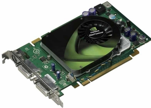
A video card, with cooling fan
