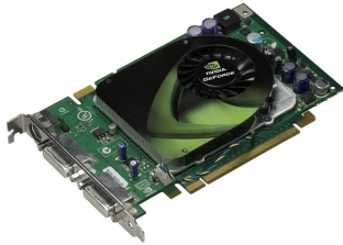
An nVidia graphics card, with cooling fan
